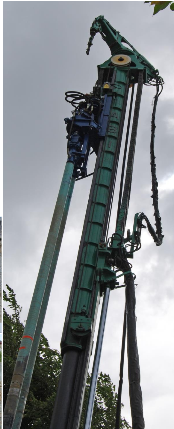
Right: Head of the high revolution auger driver.
